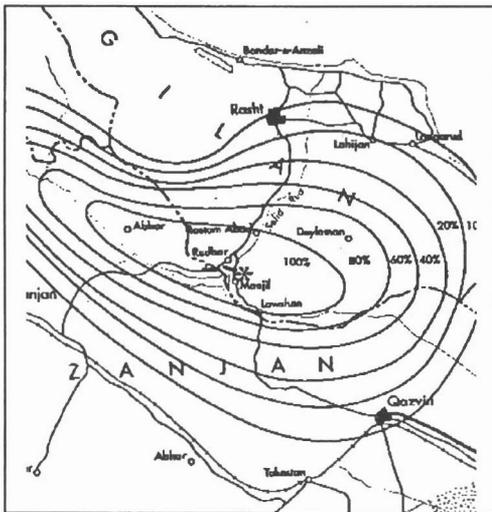
Fig. 2 Extent of structural damage
